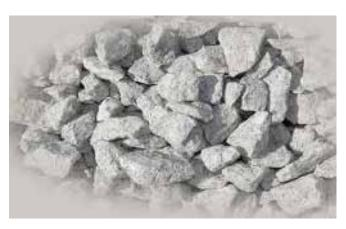
Figure 8: A sample of typical Gabion or Mattress rock.
