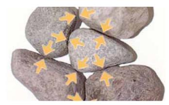
Figure 7: Diagram showing rock- on-rock contact and transfer of load at these points
